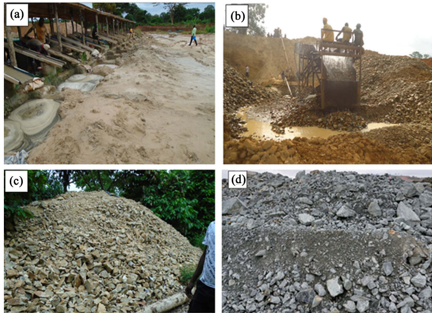
Figure 3. Types of samples taken at small mines: (a) Ore processing slurry; (b) Discharges from alluvial ore processing; (c) Bed-rock; (d) Saprolite-bedrock mixture.
