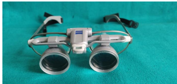
Fig. 5. Magnifying loupe 2.5 x magnification
