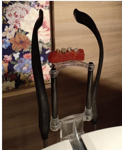
Fig. 4. 4 teeth positioned and organised in a wax slab in a row. Teeth mounted in wax blocks up to the cemento-enamel junction
