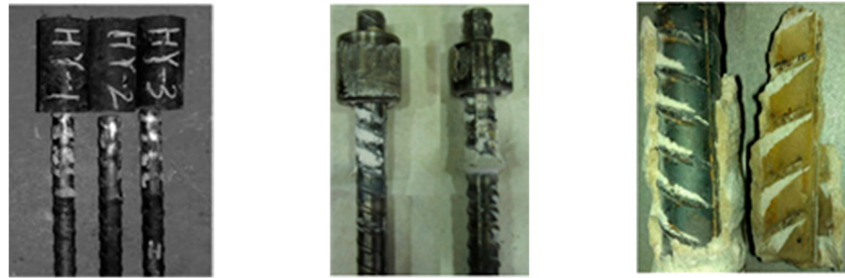
Figure 1. Interface failure of Bolt-Grout in pull-out test [3].
