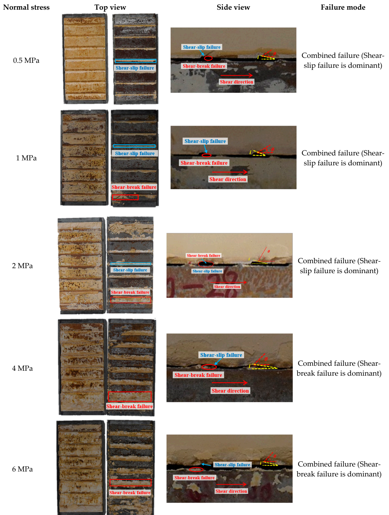
Figure 18. The failure patterns of interface under different normal stresses.
