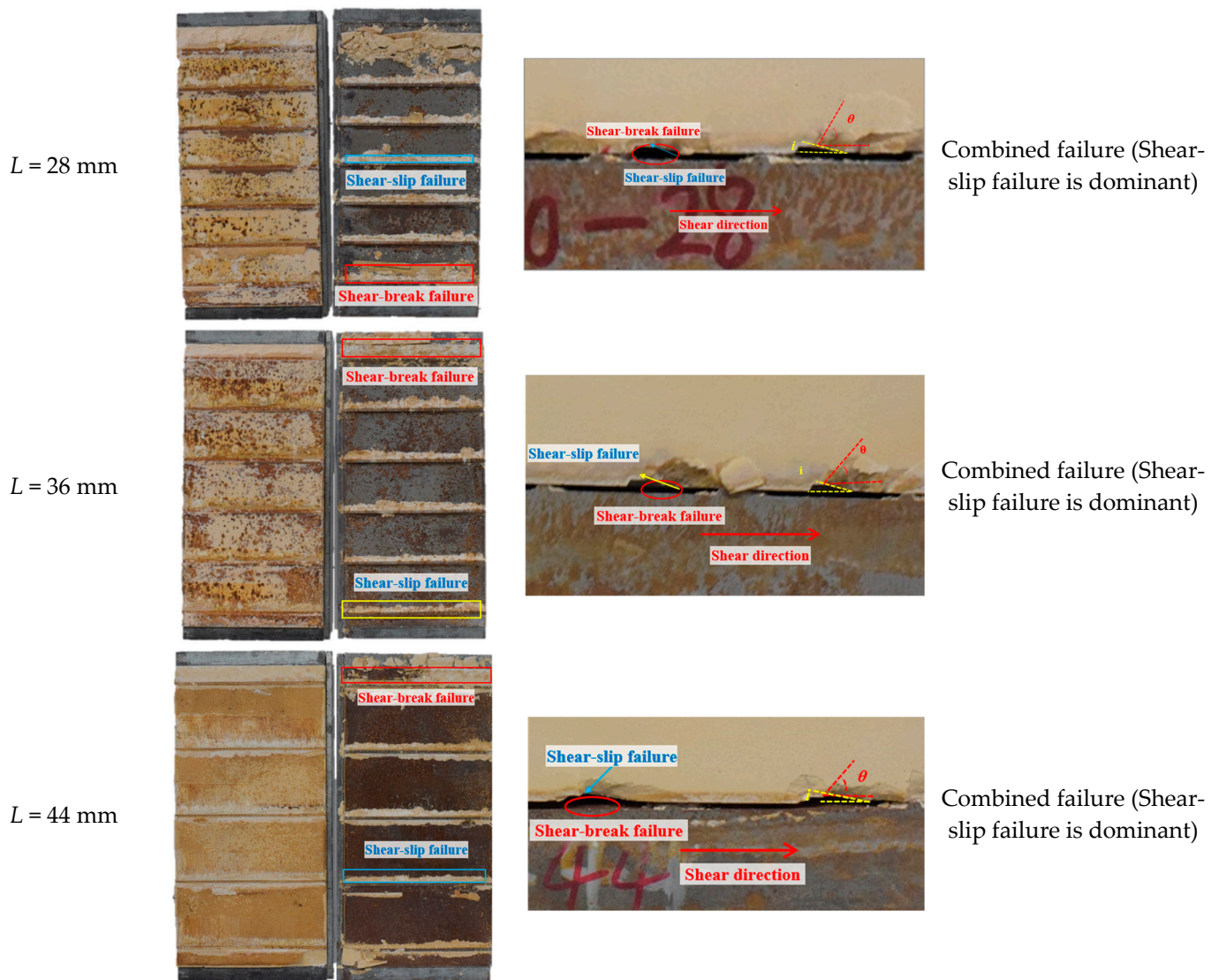
Figure 16. The failure patterns of interfaces under different rib spacing.
