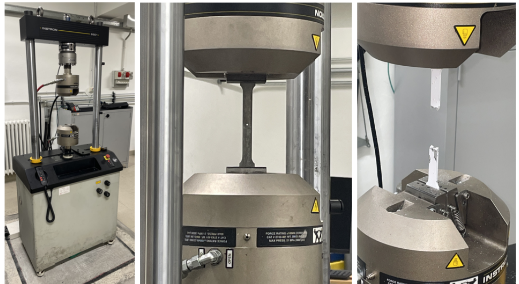
Figure 4. Specimen installed in the fatigue test machine.
