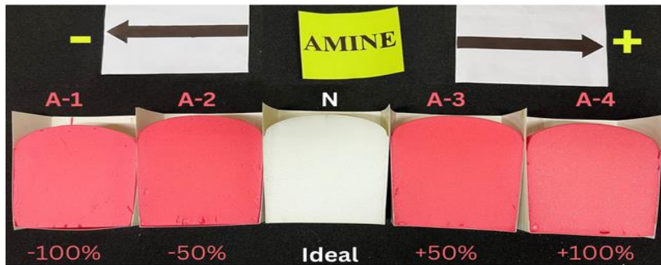
Fig. 6b. A visual illustration of the impact of varying amine concentrations on the quality of eventual flexible polyurethane foams
