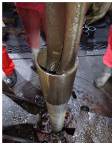
Figure 1. Crushed tubing in an oil well.
