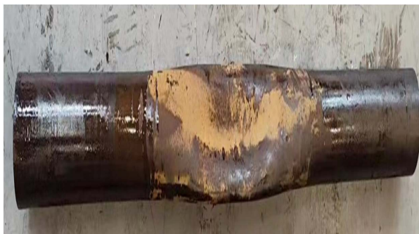
Figure 10. Collapse failure of intact tubing.
