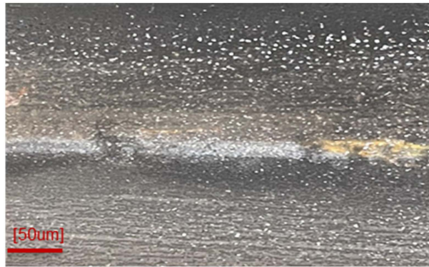
Figure 8. Macroscopic morphology of local corrosion on the inner wall of extruded tubing.
