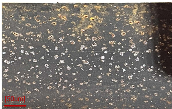
Figure 7. Macroscopic morphology of local corrosion on the inner wall of intact tubing.
