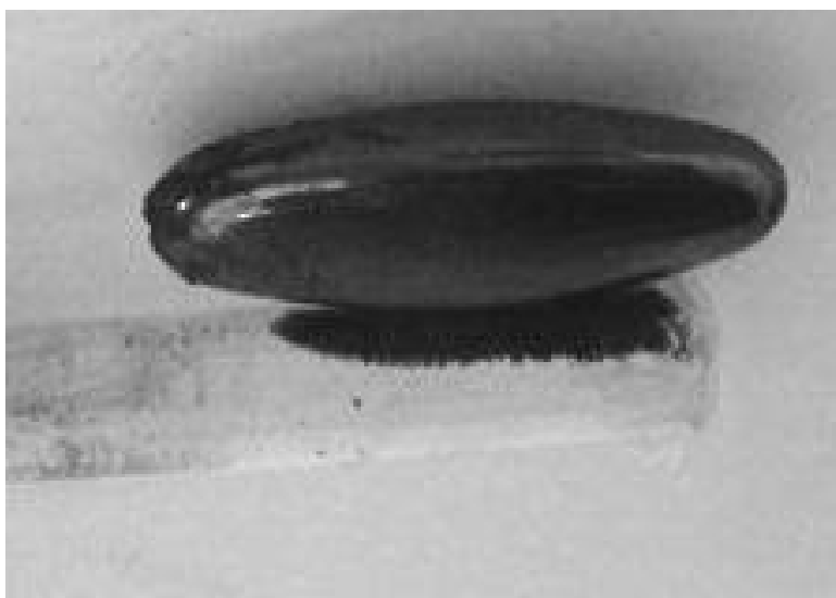
Fig. 1. Fe 3 O 4 NPs separated by a magnet
