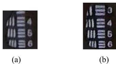
Figure 21. Panoramic images: (a) through direct image stitching, (b) through blurring, sharpening, and stitching.
