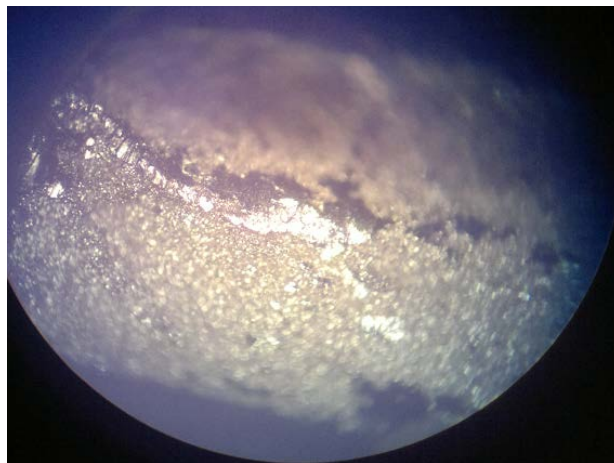
Figure 8. Black deposition on the end of a chopped alloy stick (80× optical magnification).
