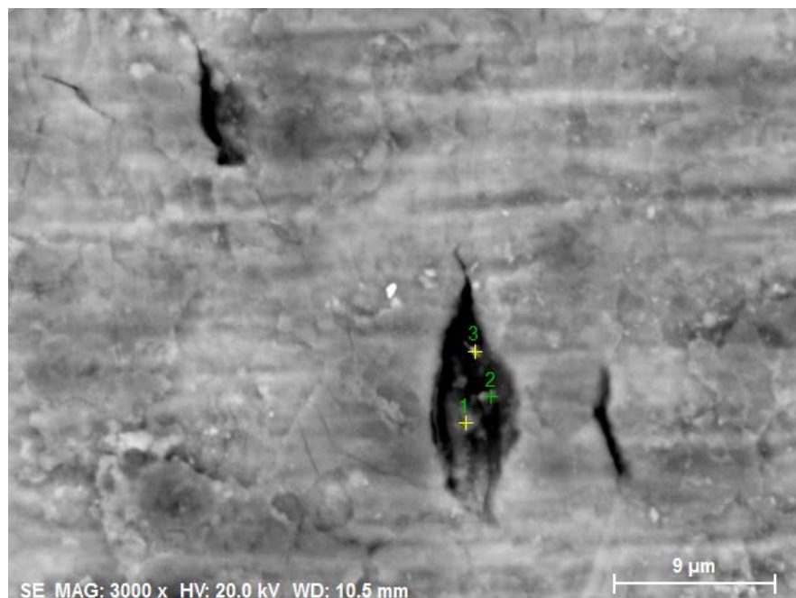
Figure 11. EDS points in the crack on Sample 2.
