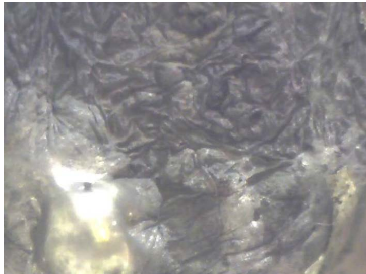
Figure 5. Carbon particles on the surface of Sn:Bi alloy (app. 150× optical magnification).
