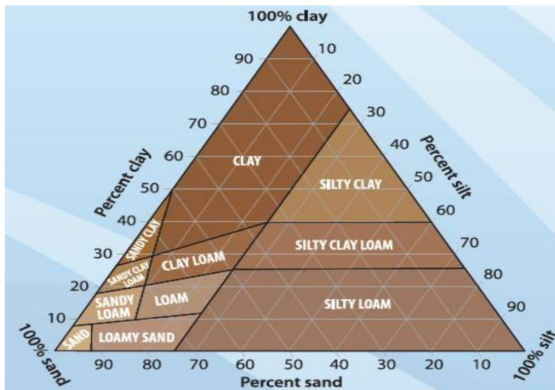
Fig. 2. Triangle of soil texture used to classify soil samples
