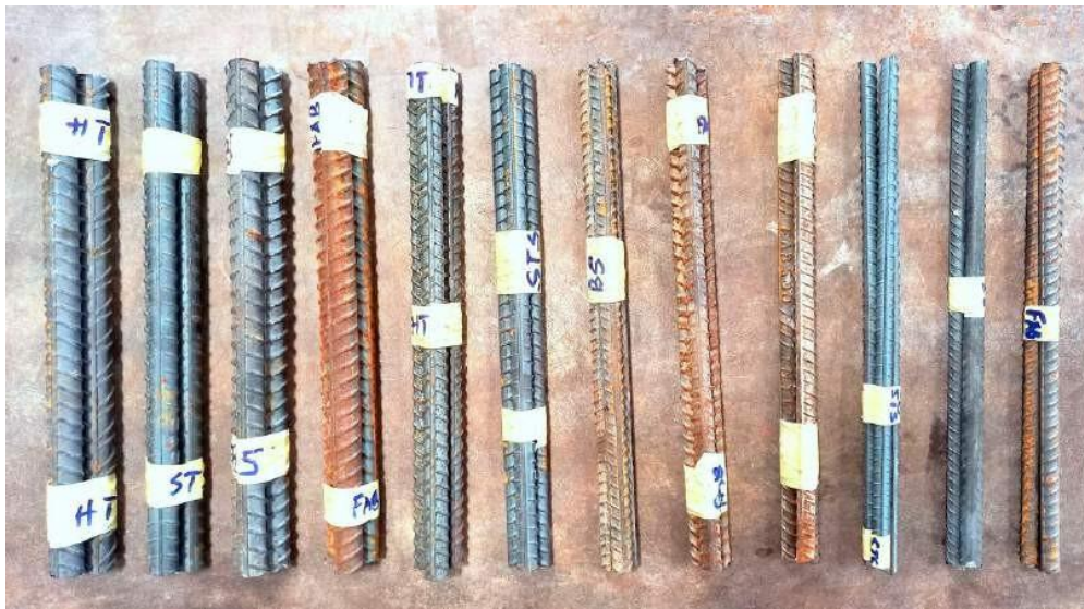
Fig. 3. Samples of the Reinforcements Prepared for the Mechanical Properties Test
