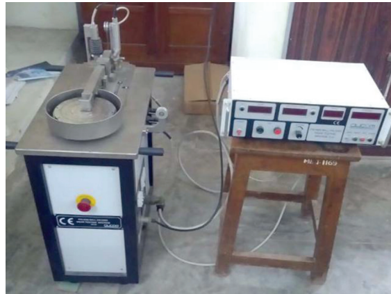
FIGURE 7: Pin-on-disc tribometer setup.
