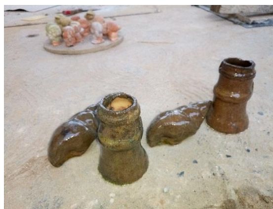
Fig. 9. Results of added feldspar to slip
