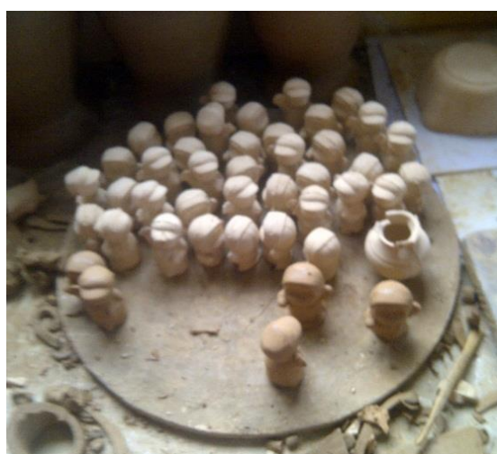
Fig. 2. Cast ceramic pieces for the glaze testing
