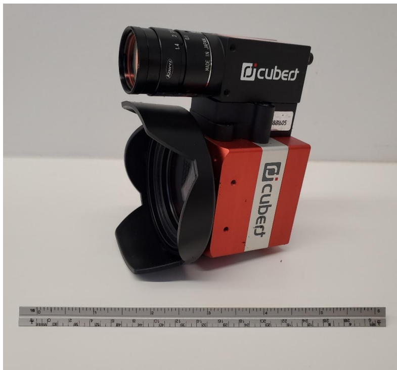
Fig. 1. Cubert ULTRIS X20 plus hyperspectral sensor. Ruler is approximately 16.5 cm in total length
