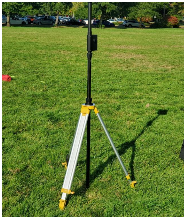
Fig. 3. DJI D-RTK 2 high precision GNSS mobile station
