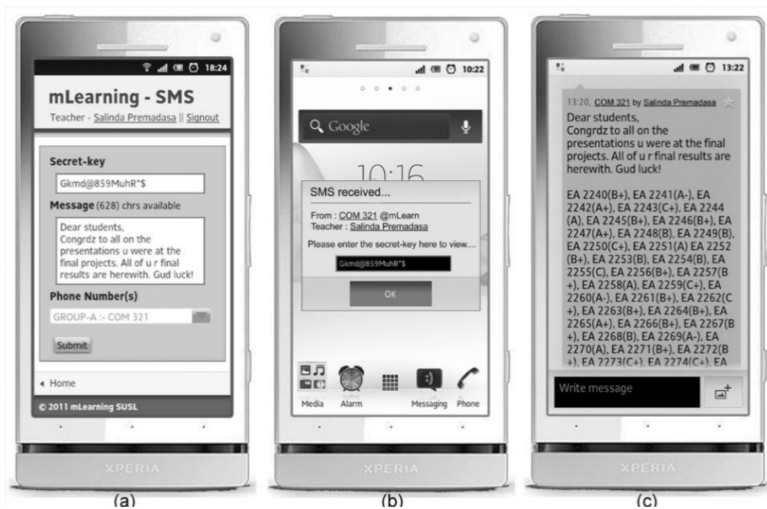
Fig. 3. Front-end interfaces of the proposed system of the mobile phone with, (a) teacher inserts extensive text message with a secret key, (b) student receives the message and inserts secret-key, (c) student views the original message
