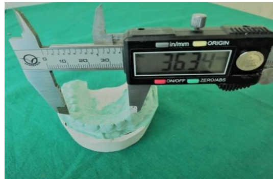
Fig. 3. Measuring maxillary intercanine width In cast with digital vernier caliper
