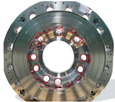
Figure 1. Image of cylinder head for large bore marine engines with 24 optical access ports (marked by red circles). Reproduced with permission from John Hult, MAN Energy Solutions.
