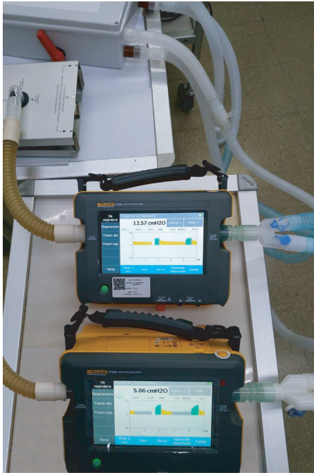
FIGURE 2: The experimental model: a ventilator connected through the DuplicAR ® device to two gas flow analyzers and their respective test lungs.
