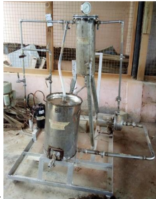
Plate 1. Chemical Impregnating Equipment used
