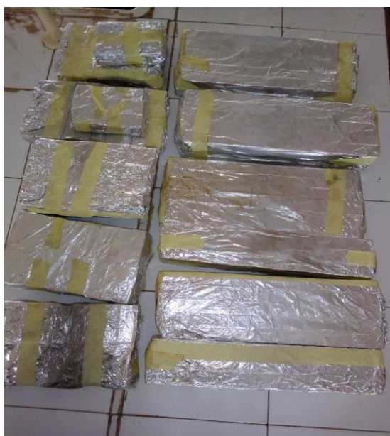
Plate 2. Treated wood wrapped with aluminium
