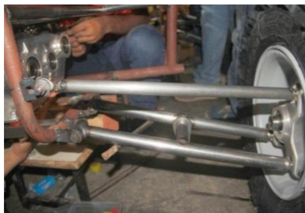
Fig. 26. Assembly of H-arm, lateral link, hub and upright
