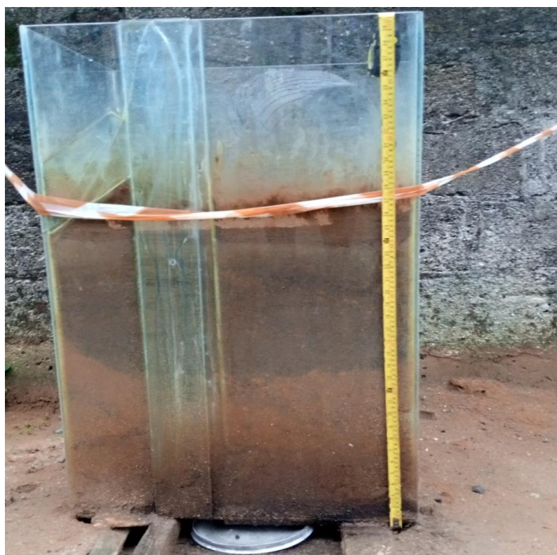
Plate 1. A graduated glass sheet of rectangular shape of soil profile (100 cm x 50 cm x 50 cm)
