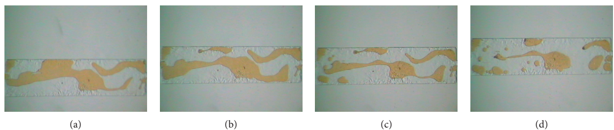
FIGURE 11: Distribution of residual oil after displacement with different Dh (pore-throat ratio 7.0). (a) Water flooding. (b) Dh = 159.7 nm. (c) Dh = 301.4 nm. (d) Dh = 327.8 nm.
