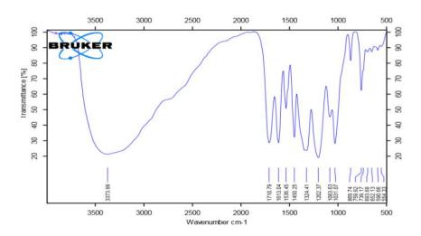
Fig. 4a. Fourier Transformed Infrared Spectroscopy of Quercus infectoria plant extract
