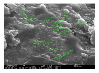
Fig. 2b. SEM image of AgNPs from D. carota
