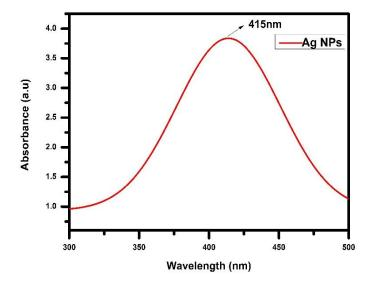
Fig. 1a. UV- Vis Spectra of synthesized Silver nanoparticles of Q. infectoria
