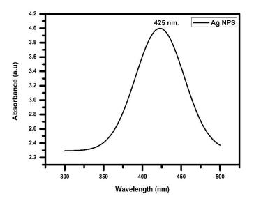
Fig. 1b. UV- Vis spectra of synthesized Silver nanoparticles of D. carota
