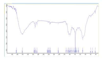
Fig. 4b. Fourier transformed infrared spectroscopy of AgNPs of Quercus infectoria
