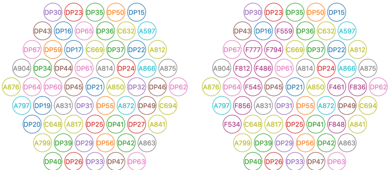
Figure 2. X441 (left) and X441A (right) subassembly layout [4].
